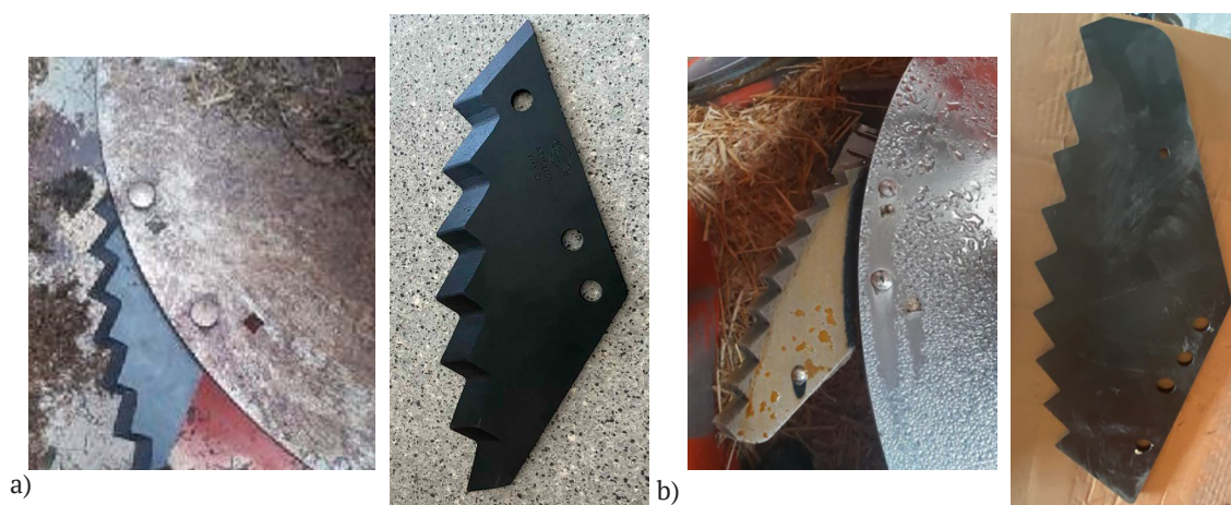
Figure 4. Knives of the PROFILE 12.2 DS and PROFILE 14.2 DS feed mixers in operation and assessment of their technical condition
