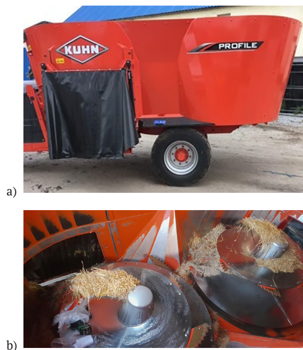
Figure 1. PROFILE 14.2 DS feed mixer (a) and chopping and mixing mechanism (b)
