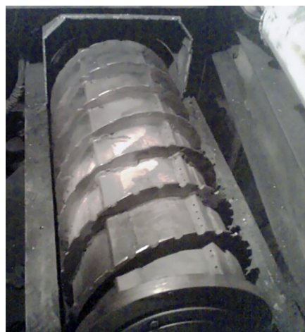
Figure 5. Operation chamber of the electric auger unit for shredding and pyrolysis of plant waste biomass (upper part of the housing removed)
