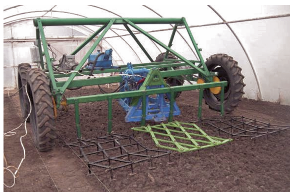
Figure 2. Laboratory for testing a new construction bridge agricultural machine with a permanent technological track
