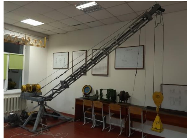
Fig. 4. Physical model of the jib crane rotation mechanism
