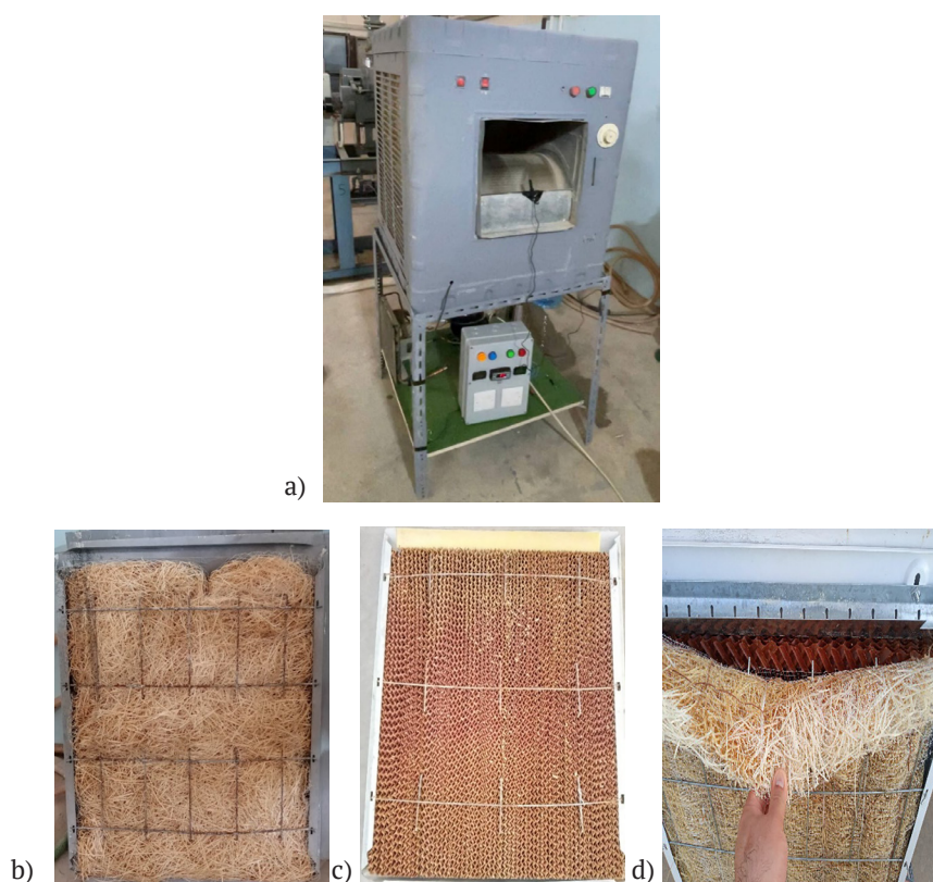
Figure 1. Types of evaporative cooler system pads
