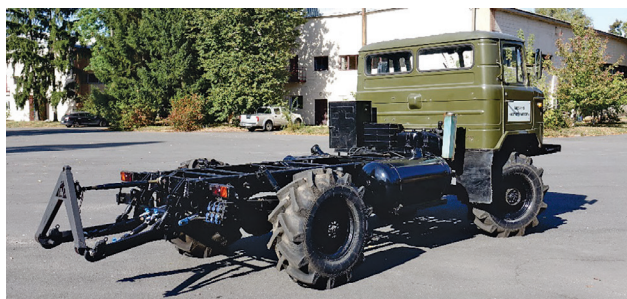
Figure 1. Mobile Energy Vehicle MEV-115 “Autotractor”
