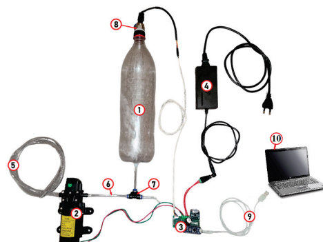
Figure 3. The structure of the experimental stand for determining the loading characteristics of the water pump
