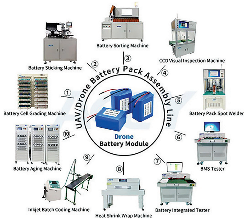
Figure 2. Technological equipment for battery production
