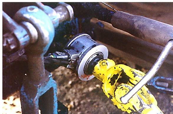
Figure 6. Load cell for measuring the angular speed of rotation of cleaning shafts
