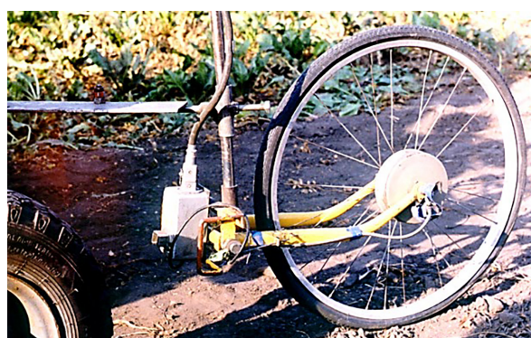
Figure 7. The track wheel mounted on the cleaner
