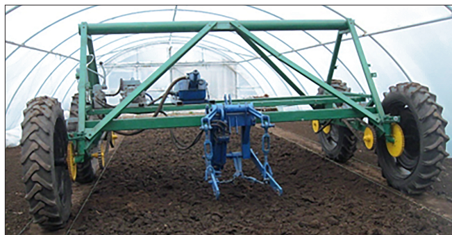
Figure 1. Experimental bridge machine
