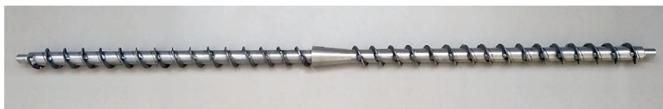
Figure 1. The screw of an electromechanical hydrolyser
