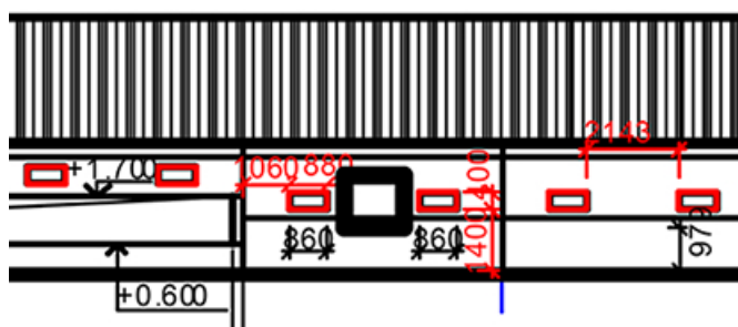
Figure 3. Location of the first exhaust fan on the side wall
