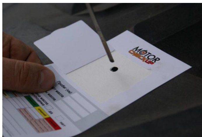
Fig. 3. Experienced application of tracer test for engine oil.
