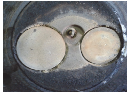
Fig. 5. Application of purified biogas as the fuel – no destruction and corrosion effects are visible
