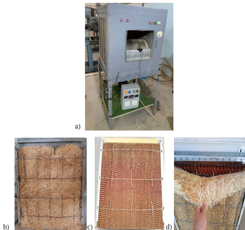
Figure 1. Types of evaporative cooler system pads
