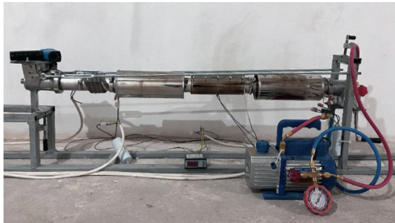
Figure 3. Screw electromechanical hydrolyser
