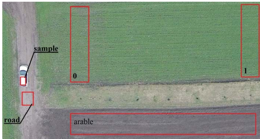
Fig. 1. The experimental department's photo with the designation of areas: where: 0 and 1 – parts with wheat sowing without and with the recommended dose of fertilizers accordingly; arable– arable seedbed; road – dirt road (air-dry condition); sample – artificial optical pattern.
