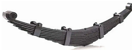
Figure 7. Leaf type spring
