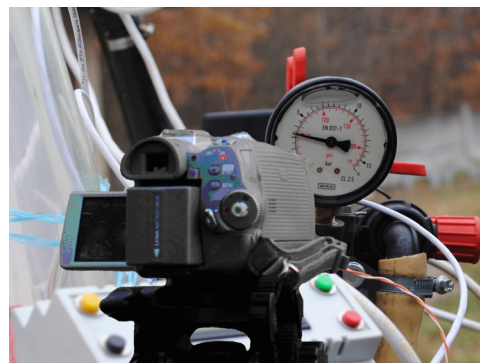
Figure 2. Recording the readings of the WIKAI EN837-1 pressure gauge when raising and lowering the pressure in the pipe
