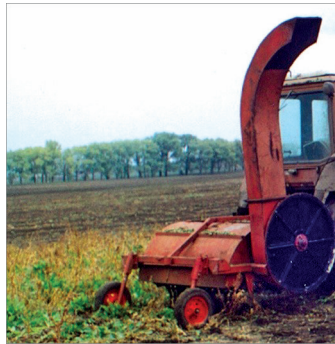
Figure 1. Root crop peeling machine with rotary cutting unit
