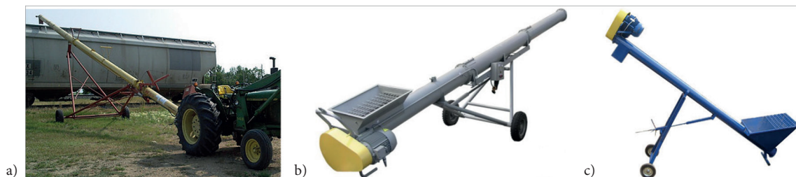
Figure 1. Hopper-fed screw conveyors: a) tractor PTO drive; b) and c) mobile screw conveyors
