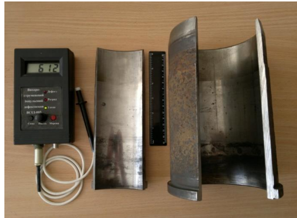
Fig. 1. Portable eddy currents pulse defectoscope (beside to the cut piece of tractor engine sleeve with the main crack on the inner surface).
