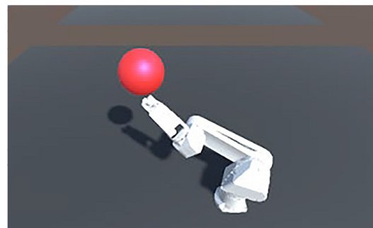
Figure 5. Using the Unity3D environment to model the movements of a robot arm
