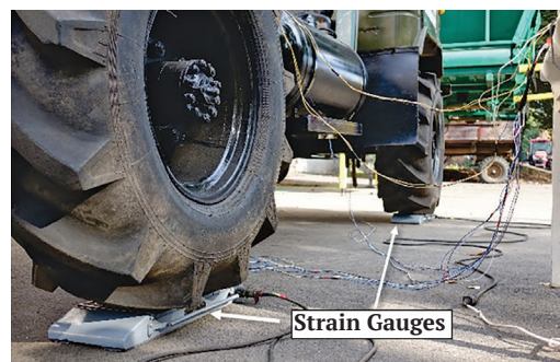
Figure 4. Placement of strain gauges on the MEV-115 “Autotractor”
